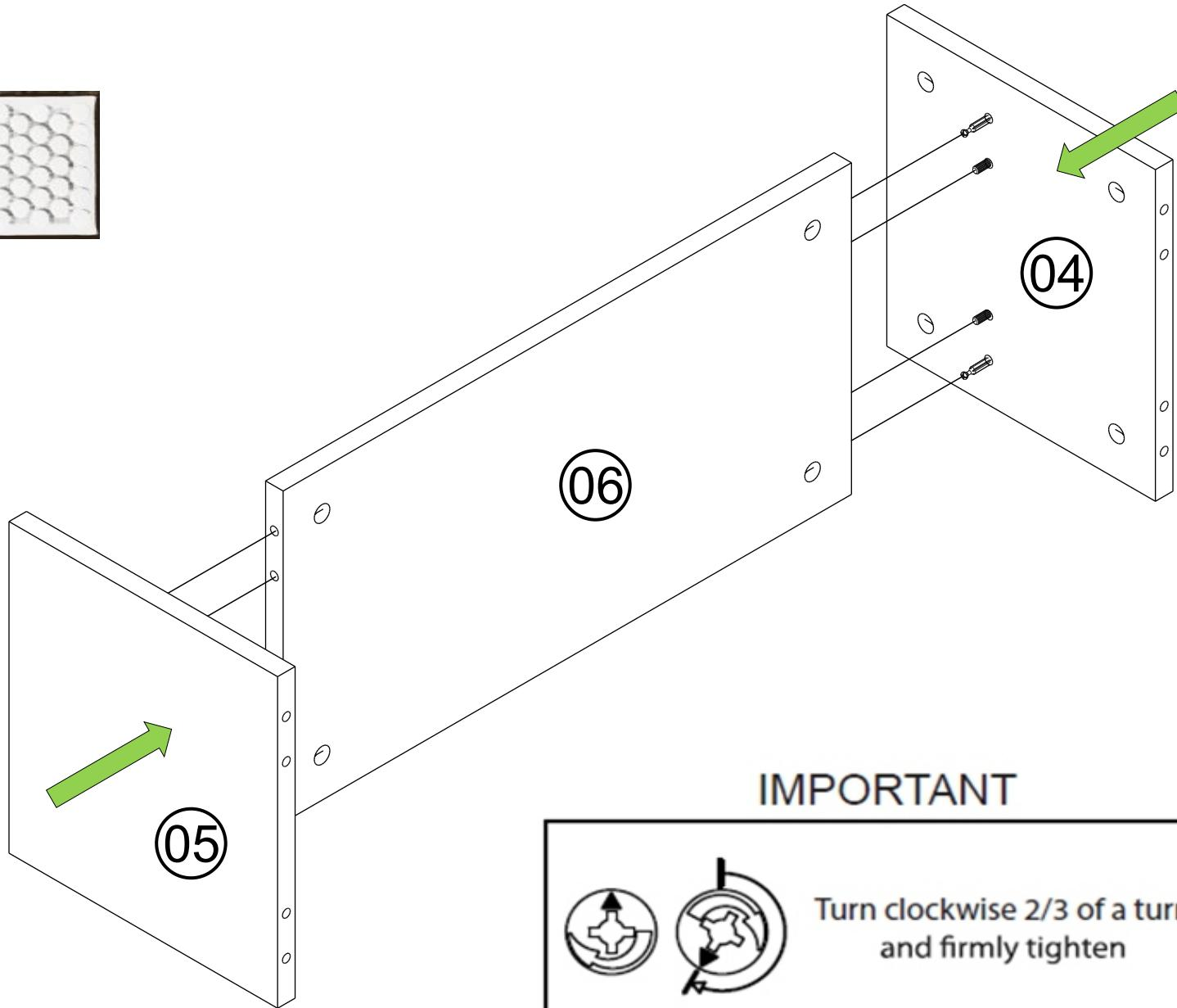
**6** Fasten the panel 3,4 and 5 to the panels 1 and 2. Then tighter the 16 cam locks.
